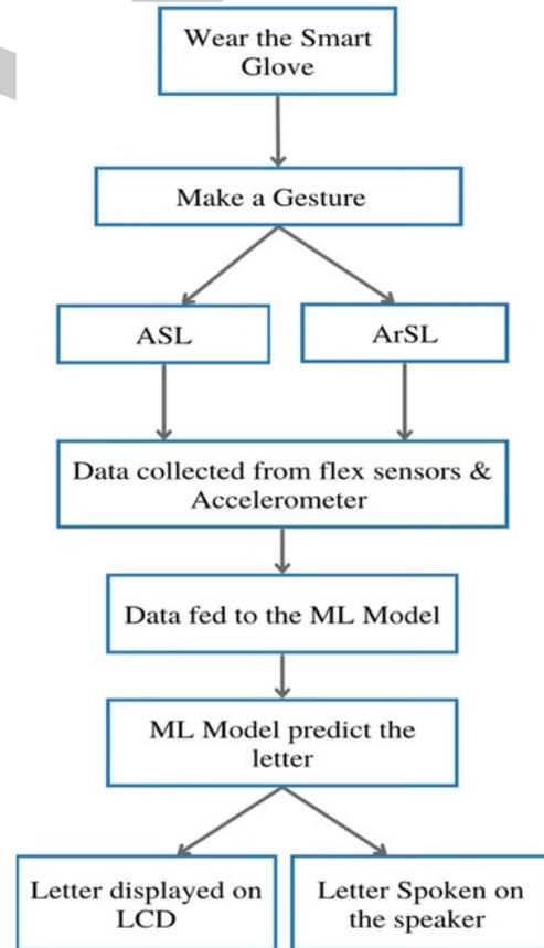
Fig. 2. Proposed smart glove approach for ASL and ArSL using ML
