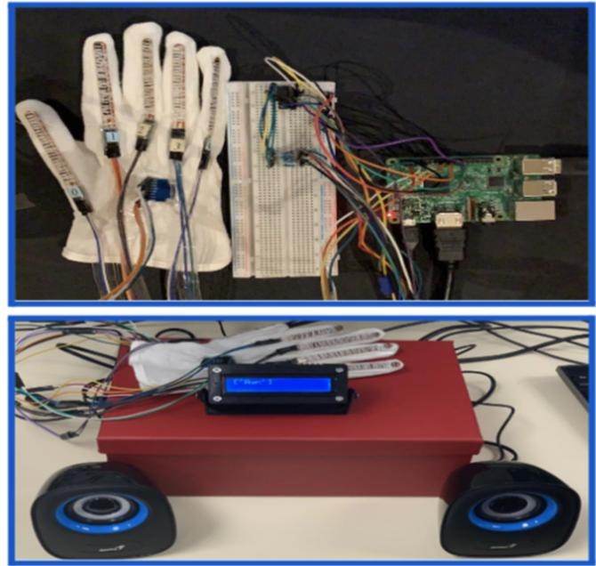
Fig. 5. Prototype implementation with Flex sensors, Accelerometer, LCD and Speakers
